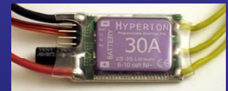
Above: electronic speed controllers (ESCs) for brushless motors: Schulze Future (top), Kontronik Jazz (middle), Hyperion (bottom)
