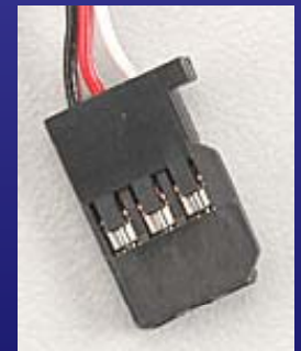
Above: servo connectors: JR/Hitec/Airtronics male connector (top); Futaba male connector (bottom)
