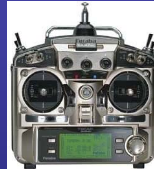
Above and to the right: radio transmitters: Futaba 9CH 72MHz transmitter (top left), JR XP9303 72MHz transmitter (top right), Spektrum DX7 DSM2 2.4GHz spread spectrum transmitter (bottom right)
