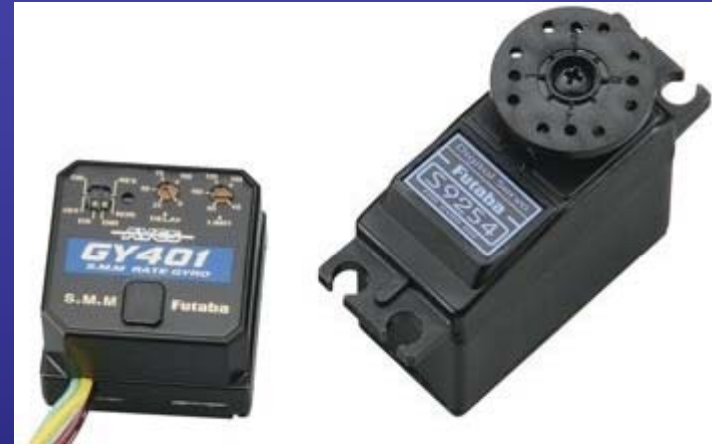
Futaba GY401 gyro with S9254 servo (top), JR G3703D gyro with DS3500G servo (bottom)
