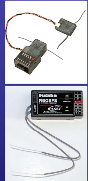
Above: 2.4GHz spread spectrum receivers: Spektrum AR7000 (top), Futaba R608FS (bottom)
