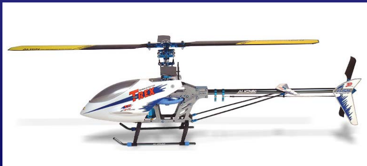
Above: Align T-Rex 450 SE electric mini helicopter with a belt-driven tail
