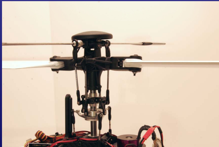
Above: Mikado Logo 10 Carbon rotor head (Photo by W. Witt)
