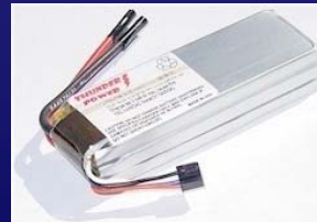
Left and below: motor batteries: Apogee lithium polymer (LiPo) batteries (left), Thunder Power LiPo battery (middle), Nickel Metal-Hydrate (NiMH) battery pack (right)
