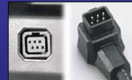
Left: Trainer port in the back of a Futaba transmitter (left), matching connector at the end of a trainer cable (right)
