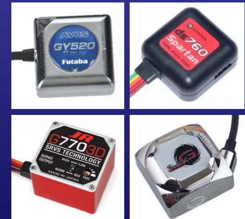
Above: high-end gyros: Futaba GY520 (top left), Spartan ds760 (top right), JR G7703D (bottom left), Curtis Youngblood Solid G (bottom right)
