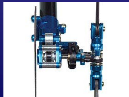
Above: Align T-Rex 600 Nitro Pro 50-size IC helicopter with torque tube drive for the tail (close up photo by W. Witt)
