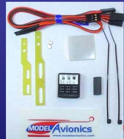
Above: Speed governors for IC helicopters: Futaba GV1 governor (top, shown here without associated sensor), Model Avionics Throttle Jockey Pro governor (bottom, with sensor and accessories)
