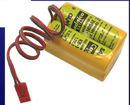
Four-cell NiCd receiver packs in a flat (left) and square configuration (bottom).
