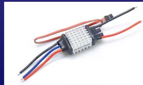
Bottom: Century Electron 50/77A ESC (left) and 80/100A ESC (right)
