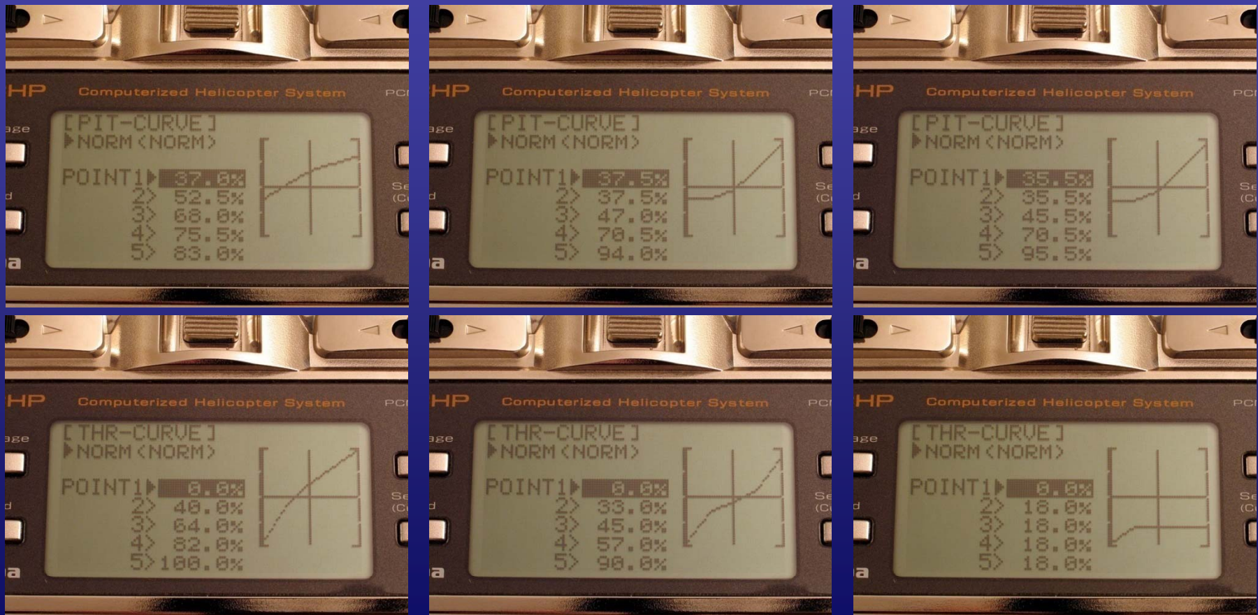
Futaba T9CHP transmitter: Pitch and throttle curve pairs for three different helicopters (left to right); the right-most curve pair is for an electric helicopter with an ESC that is running in governor mode (Photos by W. Witt)
