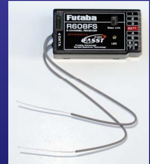
Above: 2.4GHz spread spectrum receivers: Spektrum AR7000 (top), Futaba R608FS (bottom)
