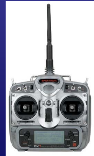
Above and to the right: radio transmitters: Futaba 9CH 72MHz transmitter (top left), JR XP9303 72MHz transmitter (top right), Spektrum DX7 DSM2 2.4GHz spread spectrum transmitter (bottom right)
