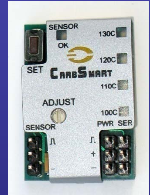
Above: CSM CarbSmart with LEDs for temperature setting on right side (100°C to 130°C)
