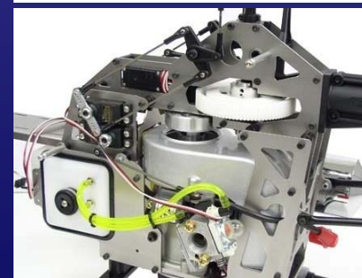
Century Predator Gasser helicopter top and to the left. Zenohu Z231HB gasoline engine middle right.
