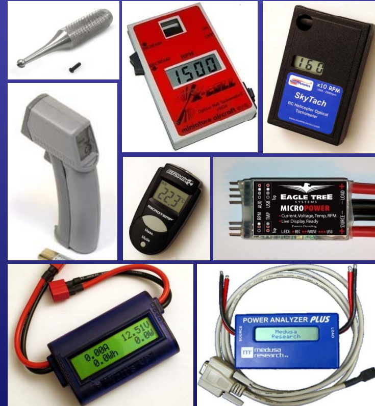
Above: ball link sizing tool from JR or Century (top left), Miniature Aircraft rotor tachometer (top middle), Model Avionics tachometer (top right, photo by W. Witt), thermometers (middle left and center), Eagle Tree Micro Power data logger (middle right), RC Electronics' Watt's Up power meter (bottom left, photo by W. Witt), Medusa Research Power Analyzer power meter (bottom right)
