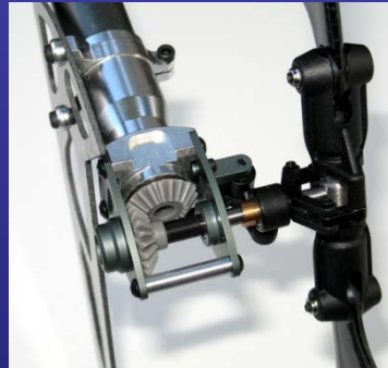
Above: Align T-Rex 600 Nitro Pro 50-size IC helicopter with torque tube drive for the tail (close up photo by W. Witt)
