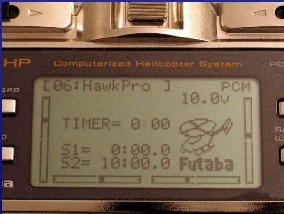
Futaba T9CHP transmitter: Primary screen showing select model (HawkPro), digital trims and timers (left); basic programming menu (middle); advanced programming menu (right) (Photos by W. Witt)
