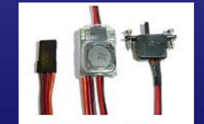
Above: switching voltage regulators (top to bottom): Castle Creation's BEC, Kool Flight System's Ultimate BEC and micro Ultimate BEC, SBEC
