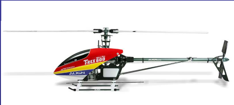
Above: Align T-Rex 600 Nitro Pro 50-size IC helicopter with torque tube drive for the tail (close up photo by W. Witt)
