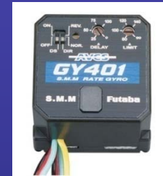
Above: Futaba GY401, a very popular mid-range gyro (heading hold or rate mode)
