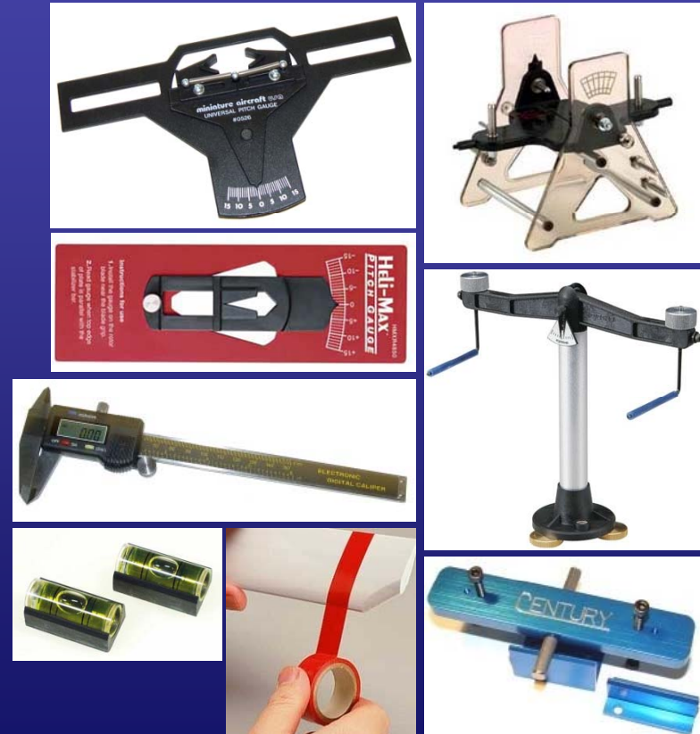
Above left (top to bottom): Miniature Aircraft main rotor blade pitch gauge, Heli-Max pitch gauge, digital caliper, small bubble levels, Heli-Max blade tracking tape
