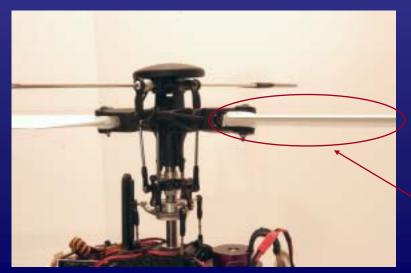
With increasing collective pitch, the leading edges of the rotor blades angle up for more lift.
