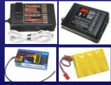
Futaba R149DP (top left), JR R2000 (top right), HiTec Electron 6 (bottom left), typical 4-cell NiCd receiver battery (bottom right)
