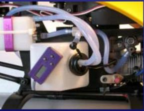
Above: Main tank and header tank installed in a Century Hawk Sport helicopter (top); main tank and header tank in a Hawk Pro (bottom). Stuck to the main tank of the Hawk Pro is an on-board temperature meter with its sensor attached to the engine (not shown).
