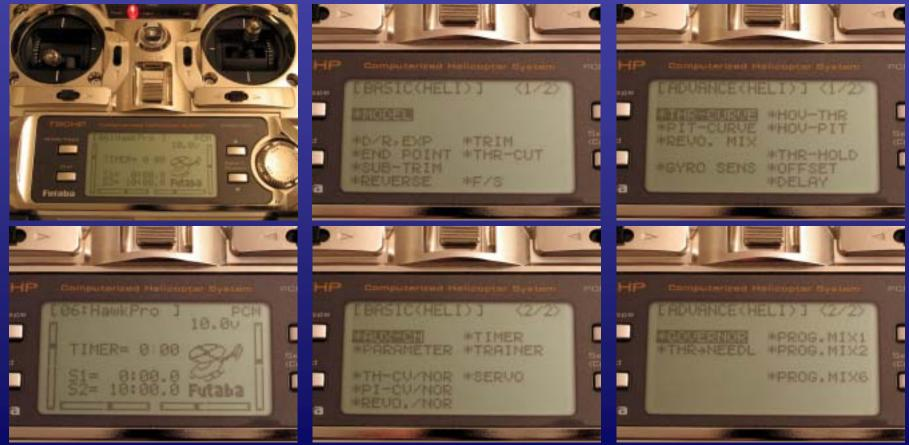
Futaba T9CHP transmitter: Primary screen showing select model (HawkPro), digital trims and timers (left); basic programming menu (middle); advanced programming menu (right) (Photos by W. Witt)
