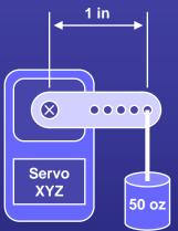
Servo Strength: A servo that can hold up to 50 oz with an arm of 1 in has 50 oz-in of holding power or torque. 50 oz-in is also equivalent to holding 25 oz with a 2 in arm, and so on. Torque values range from less than 10 to more than 200 oz-in.
