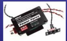
Above: linear voltage regulators: Arizona regulator from Fromeco (top), Power Force regulator from FMA Direct (bottom)
