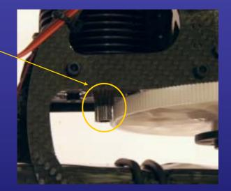
The example pictures above are from a Logo 10 Carbon helicopter. This helicopter's main gear has 200 teeth, and available pinion gears range from 13 to 23 teeth, providing gear ratios from 1:15.4 to 1:8.7.
